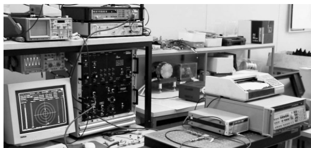
Figure 4. A view of the laboratory installation showing the MVNA (dark) in the middle, the DDS generator and the time-base generator to the right. The microwave counter is on top of the shelf.
